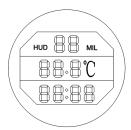
To use the timer function gently press the middle of the display, and the minute/seconds will blink in the display, turn the knob to select the time required, and press the display again to exit time setting. The mixer will beep and stop when the time has expired.
