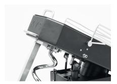
The tilt head has a handle in front, pull the handle to unlock the head and use the top handle to lift it up. If the handle is hard to pull out then apply a little downward pressure on the top while pulling the handle.
