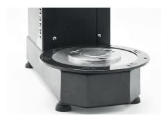
The mixing bowl sits onto the locking plate by inserting all three metal knobs into holes cut out in the plate. Turn the plate to lock or unlock the mixing bowl - the directions are shown by arrows on the plate. If the locking/unlocking is hard to do by hand, use the supplied tool to help ease the locking/unlocking.
