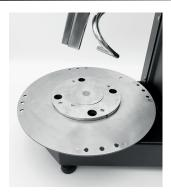
The mixing bowl sits onto the locking plate by inserting all three metal knobs into holes cut out in the plate. Turn the plate to lock or unlock the mixing bowl - the directions are shown by arrows on the plate. If the locking/unlocking is hard to do by hand, use the supplied tool to help ease the locking/unlocking.
